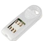
The LogicStick enables the user to program PLC functions within the drive. It can also be used as a SmartStick
